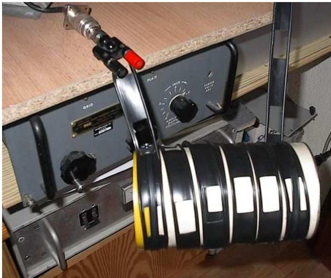
Fig.2 Example of an „airwound“ Balun
