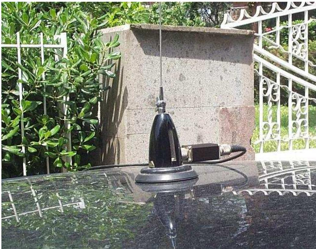
Amazingly, the circuit worked immediately and, turning the ferrite core, the SWR on 10 meters went down to nothing. Subsequently, I changed the matching network design, using a fixed coil and a variable capacitor, but this does not change the substance..
