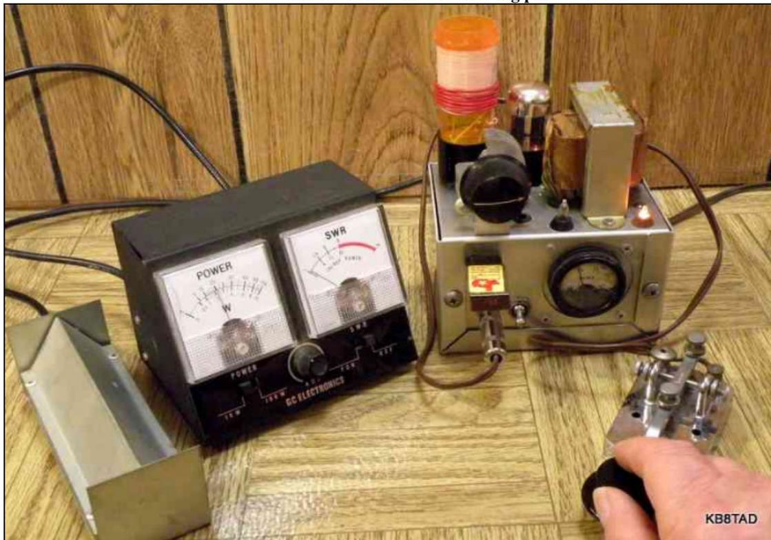
Since the difference seemed to be because the output coil was wound directly over the grounded end of the tuning coil with closer coupling, I decided to use that new 6 turn coil for the permanent output to antenna and ground. A picture of that experimental pill-bottle coil mounted on a tube base is shown above. I had the same results with both transmitters.
