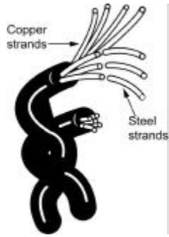
A diagram showing a bundle of seven wire strands. Four strands are labeled 'Copper strands' and are shown bending away from the other three strands, which are labeled 'Steel strands'. The steel strands are shown straight and wrapped by the copper strands. |
