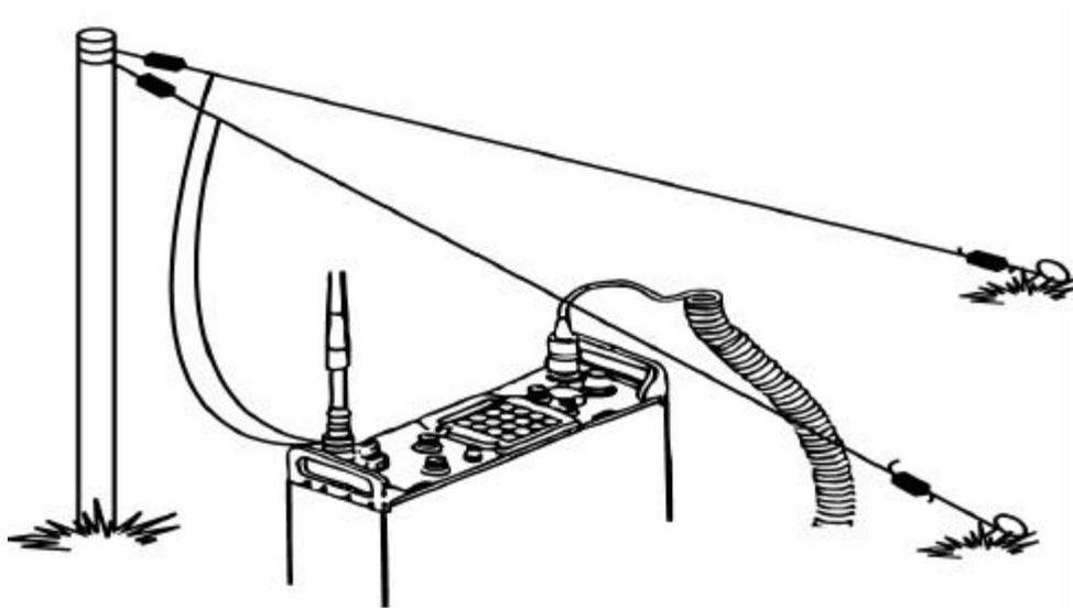
**Gain** As the leg length of this antenna increases, so does the gain. The gain (increase in effective power or performance) of a "V" antenna is almost double that of a single long wire, since the radiation from the lobes of two waves combine, reinforcing one another. To optimize this reinforcement, use the table found in Appendix A to make sure the accuracy of the apex angle (top angle where the radiating elements meet the mast section).
