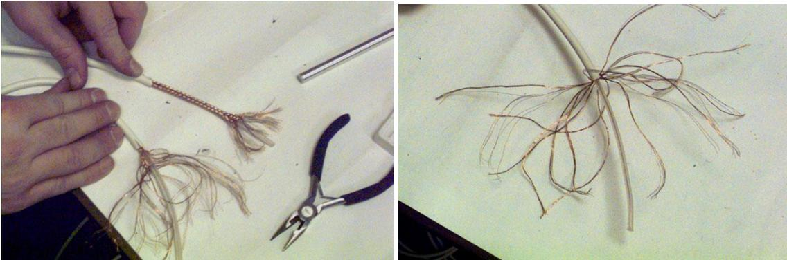
Figure 5.2a and 5.2b. Unbraid the copper shielding.
