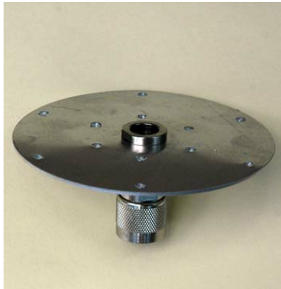
Photo 2 Ground plane radial element mounting plate assembly
