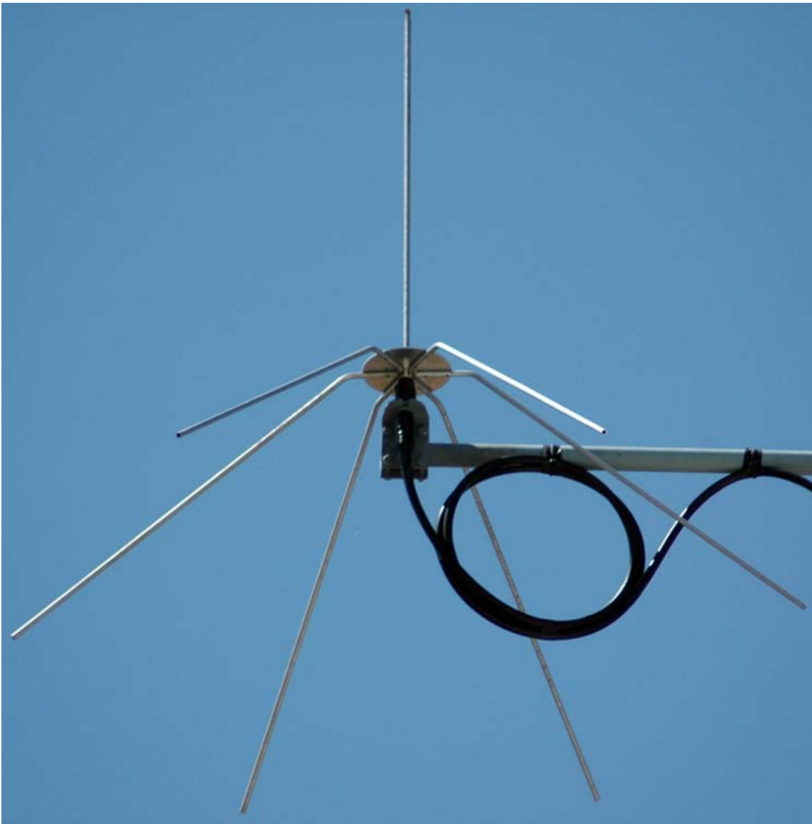
Photo 5 146MHz 1/4\lambda ground plane assembled and installed.
