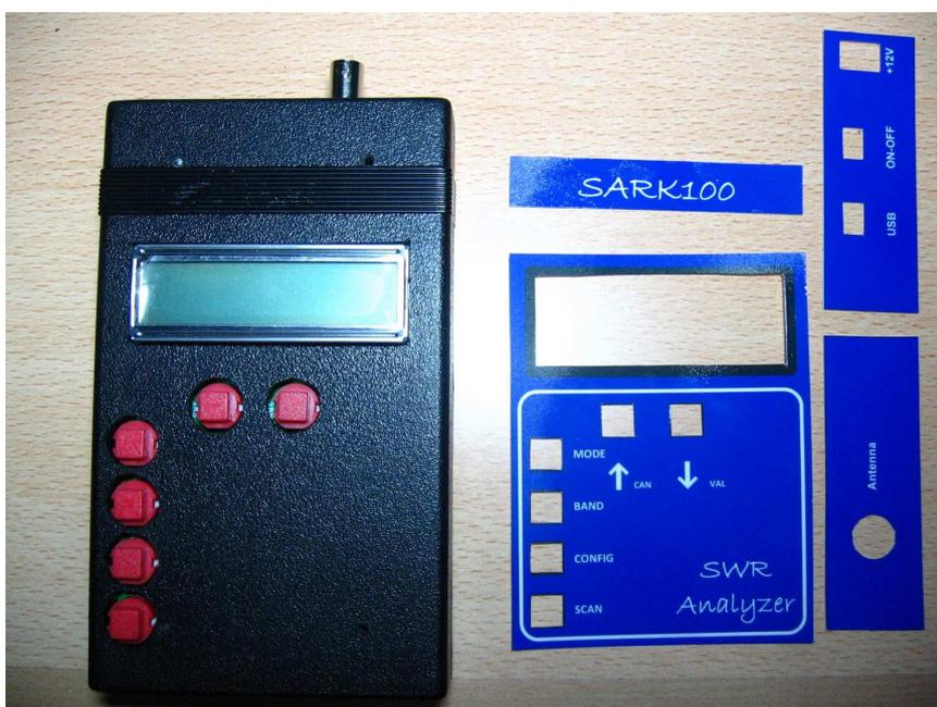
Finally, carefully paste the overlays to the front enclosure and the panels. The result must be like the following illustrations, with one sample with the box in gray and another in black.
