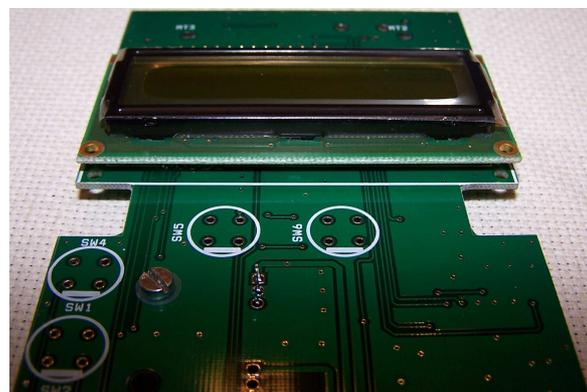
Congratulations, once it gets to this you are finished assembling the board. At this point you can optionally connect the battery holders or wait until later since you can do the power-up by connecting a power source. The battery holders are to be interconnected in series, i.e. the
