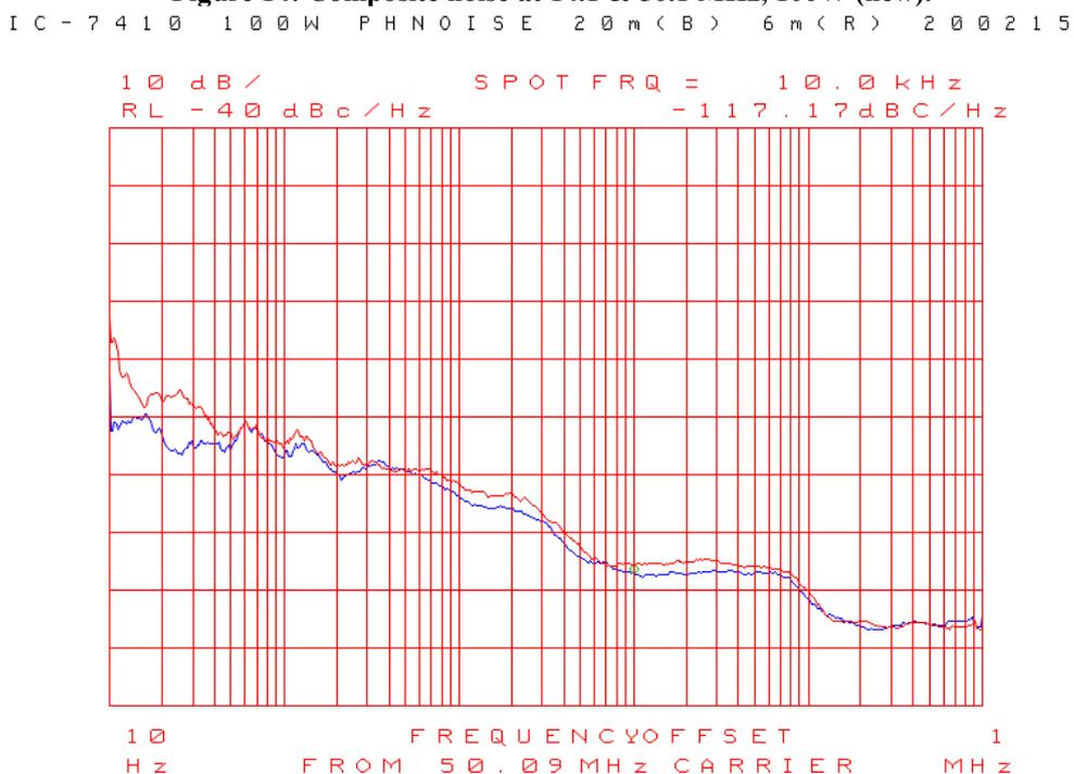
Figures 15 and 16 show the corresponding results from my original test report (2011-2012) for the same IC-7410 with the original MAIN UNIT board. Note the 100 Hz minimum offset.
