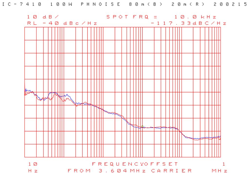
**Figure 14: Composite noise at 14.1 & 50.1 MHz, 100W (new).**
