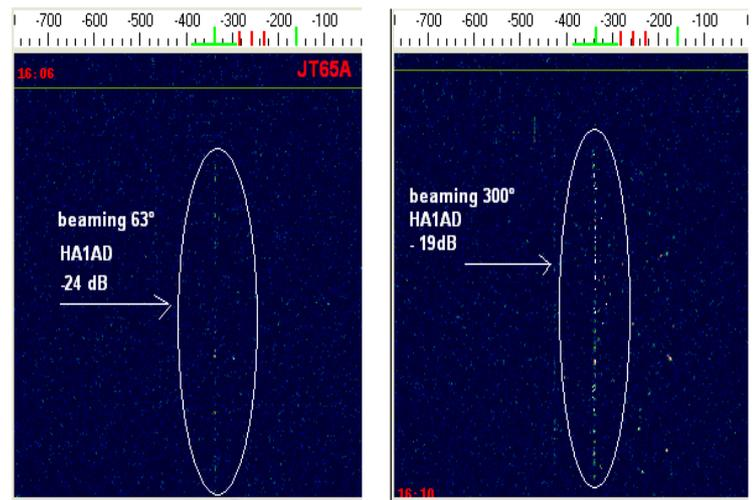
transmission wsjt in digital mode jt65a of Hungarian HA1AD station on 14076 mhz. The azimuth to Hungary is 60 ° while the signal was detected with the antenna beaming 300 °
