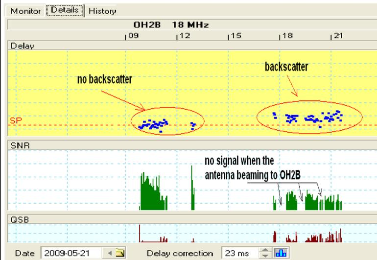
Picture Above: The faros software experiments conducted on different days always highlights the phenomenon of backscatter in the late afternoon and evening. The test conducted by alternating the reception beaming short path to the beacon and beaming Towards the area of scatter (see the graph with green colour of SNR display)
