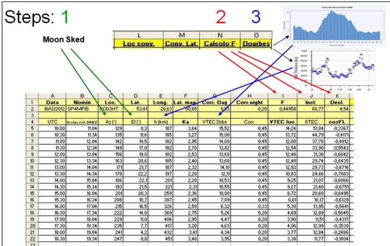
The sheet converts the ionospheric data for the station’s location, calculates the increase of ion density due to oblique passage (Ka), and finds the magnetic field component in the wave’s direction (cosFM).
