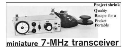
achieved by switching in a 7uh coil in series with the VXO crystal. VXO range was about 4KHz, depending upon the activity level of the crystal.
