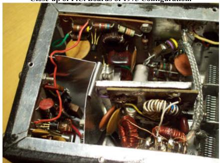
The v.f.o. p.c.b. is enclosed by a shield box at the front left, where the metal 2N706 oscillator is barely visible behind the front panel, with the 2N4124 buffer where the red output lead leaves the p.c.b. on the way to the buffer/driver p.c.b. which is mounted on
