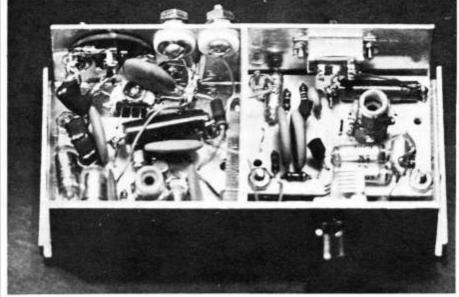
Front angle view. Shows VFO ON-OFF, Key, B+, and ANT JACK. Bolt mounting final transistor tab to box is visible between ANT and B+ post. 68pf T-R capacitor and diodes just above output toroid. Outside ANT JACK mounting screw is insulated from box, has a solder lug, and serves to connect receiver to antenna through solid-state T-R switch.
