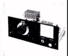
Front view of the direct conversion receiver. The panel is finished in machine gray spray paint. The two controls are main tuning and audio gain.
