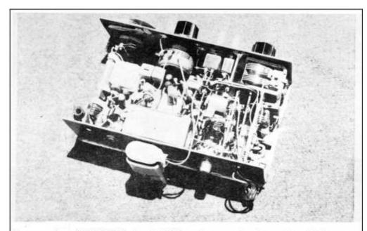
Top-rear view of WA6ZHT rig. r-l, VFO tuning capacitor front right, VFO board, shield between VFO and transmitter board, next is transmitter board; BFO and T/R switch front panel, volume control, and receiver tuning capacitor left end of volume control, and receiver tuning capacitor left end of front panel. BC receiver board left half of chassis.
