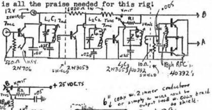
LiC1, L2C2 to tune 7mc. (180pf trimmer, 25t #24 on 3/8" slug tuned form. Links=2t on cold end. Tap set for best drive to next stage.) L3C3=to tune 14 mc. (60pf trimmer,
