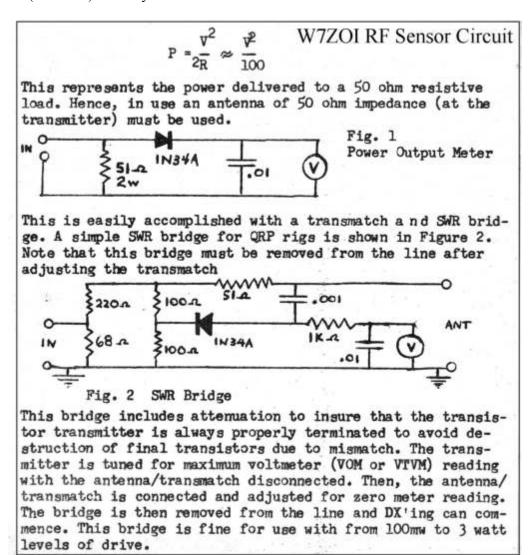
The impedance of standard VTVM and VOM devices is extremely high compared to the 50-ohm load resistor, so it does not affect the accuracy of the reading. While Hayward does not comment, the beauty of the simple circuit is that it can be accurately calibrated using a known d.c. voltage source (battery) at the input terminals of his circuit, or at the "CALIBRATION POINT" in my circuit below (from **HAM RADIO**, October, 1973, 26-29.
