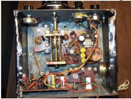
Close-up of Dual Section Variable and V.F.O. Band Module with L5-L6 and Trimmer Capacitor Beneath it.
