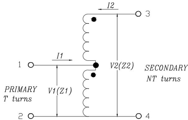
**Figure 1a** Autotransformer
