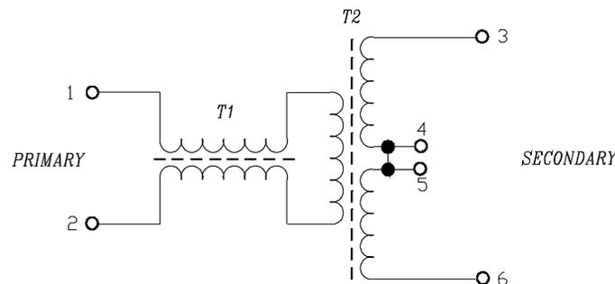
**Figure 2 High-frequency Transformer with Balun on Primary Side**
