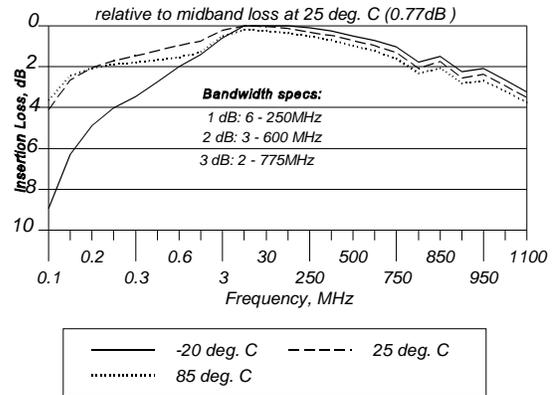
**Figure 7 Model ADT16-1T Insertion Loss**
