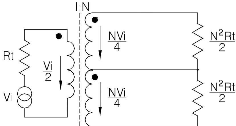
**Figure 14 - Voltage Relationships for Transformer with Matched Secondary Terminations**
