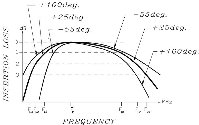
**Figure 3 Typical Frequency Response of an RF Transformer**
