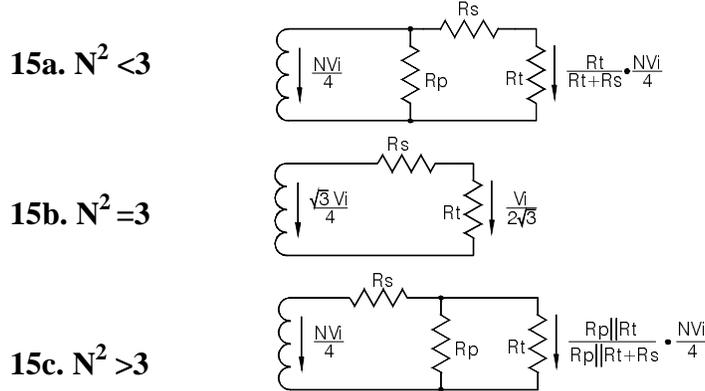
**Figure 15 Voltage Relationships for Power Calculation**
