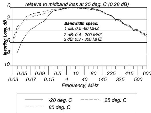
**Figure 6 Model ADT4-1WT Insertion Loss**
