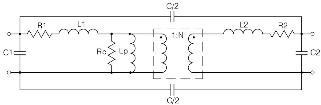
**Figure 8 - Equivalent Circuit of Transformer**
